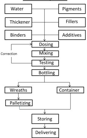
The figure shows the following working process during the production of exterior paint systems:
